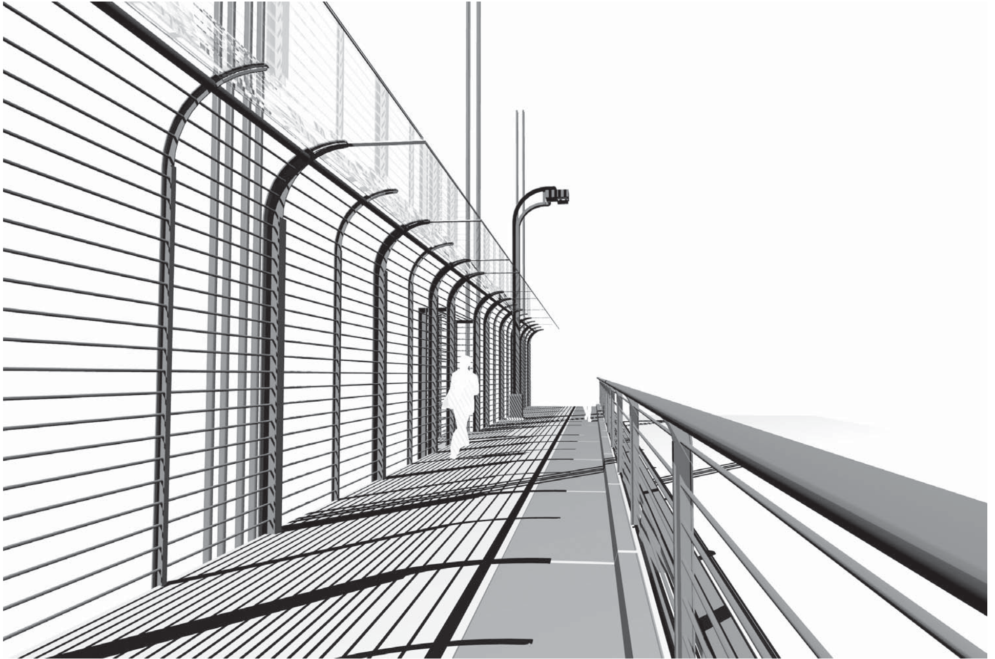
FIGURE 2.9b - EXAMPLE OF CONCEPT 2 (EXAMPLE SHOWN WITH HEIGHT OF 12'-0", 42" TRANSPARENT WINGLET, HORIZONTAL MEMBERS SPACED AT 6", SOLID RATIO OF 17%) VIEW FROM SIDEWALK
