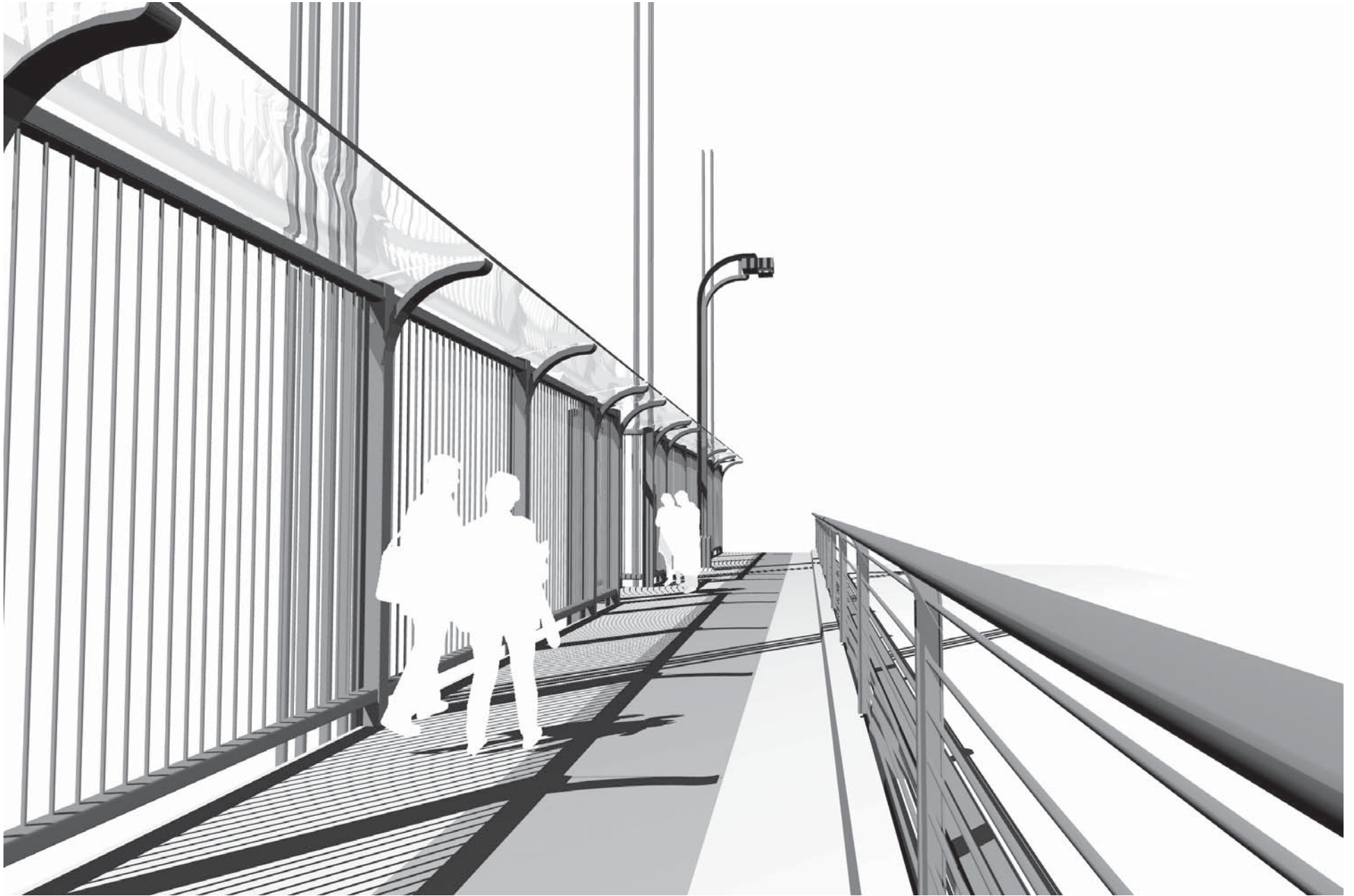
FIGURE 2.8b - EXAMPLE OF CONCEPT 2 (EXAMPLE SHOWN WITH HEIGHT OF 10'-0", 48" TRANSPARENT WINGLEET, VERTICAL MEMBERS SPACED AT 6", SOLID RATIO OF 18%) VIEW FROM SIDEWALK
