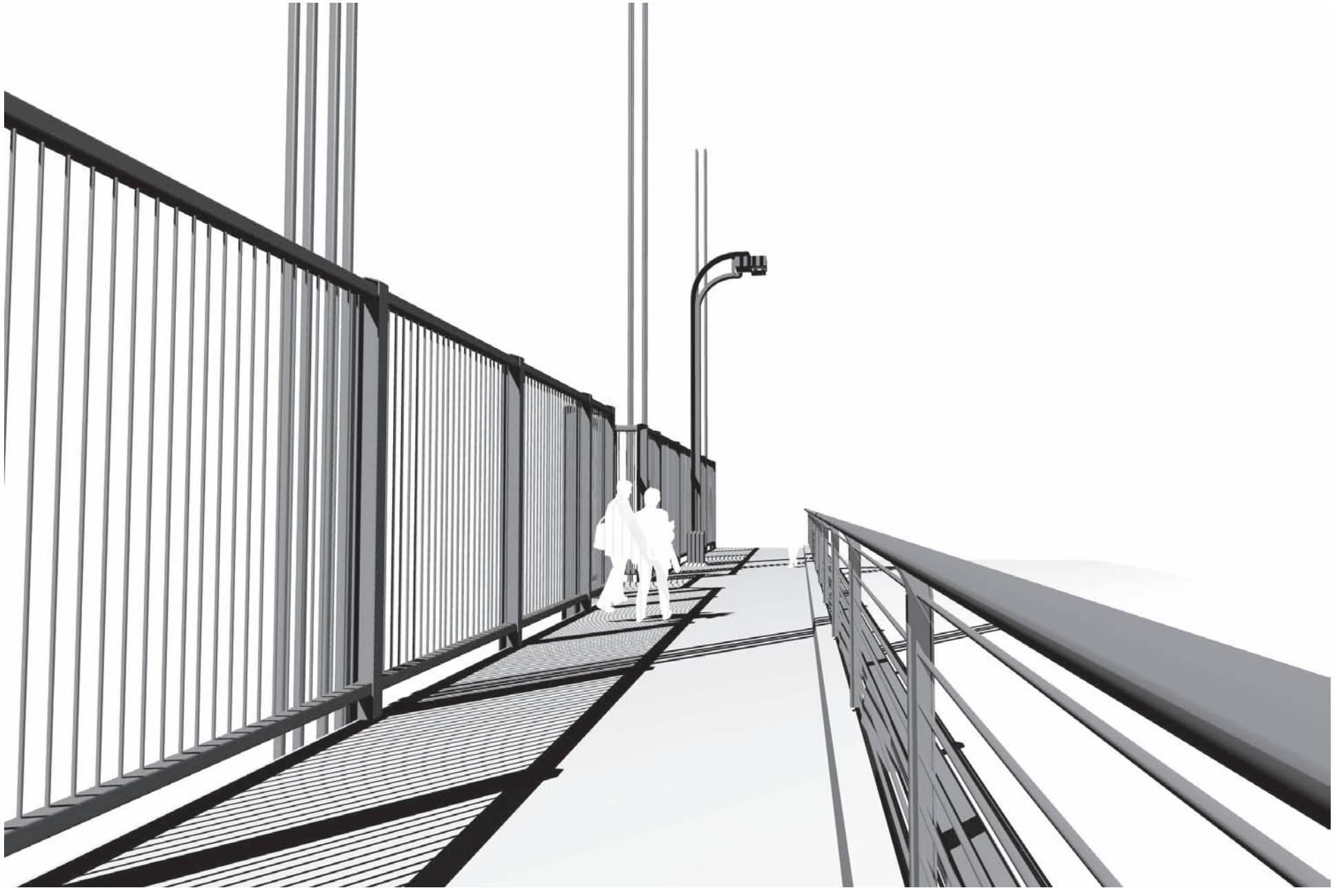
FIGURE 2.2b - EXAMPLE OF CONCEPT 2 (EXAMPLE SHOWN WITH HEIGHT OF 10'-0", NO VISIBLE WINGLET; 50" UNDER DECK WINGLET ON EAST SIDE AND 48" CATWALK ON WEST SIDE, VERTICAL ROD MEMBERS SPACED AT 6", SOLID RATIO OF 18%) VIEW FROM SIDEWALK
