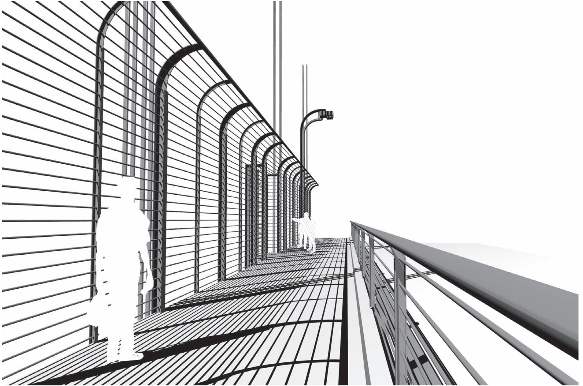
FIGURE 2.3b - EXAMPLE OF CONCEPT 2 (EXAMPLE SHOWN WITH HEIGHT OF 14'-0", NO VISIBLE WINGLET; 50" UNDER DECK WINGLET ON EAST SIDE AND 48" CATWALK ON WEST SIDE, CURVED TOP, HORIZONTAL CABLE MEMBERS SPACED AT 6", SOLID RATIO OF 16%) VIEW FROM SIDEWALK
