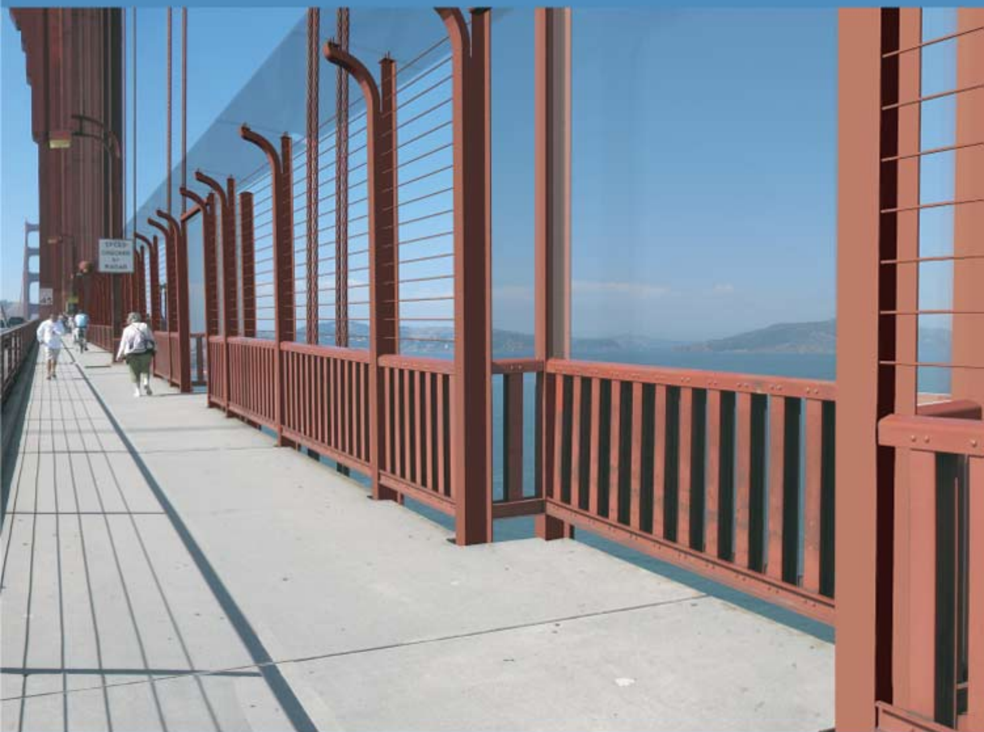
Alternative 1B - Adds 8-foot-tall horizontal system to 4-foot handrail, with winglet on top Sidewalk View North
